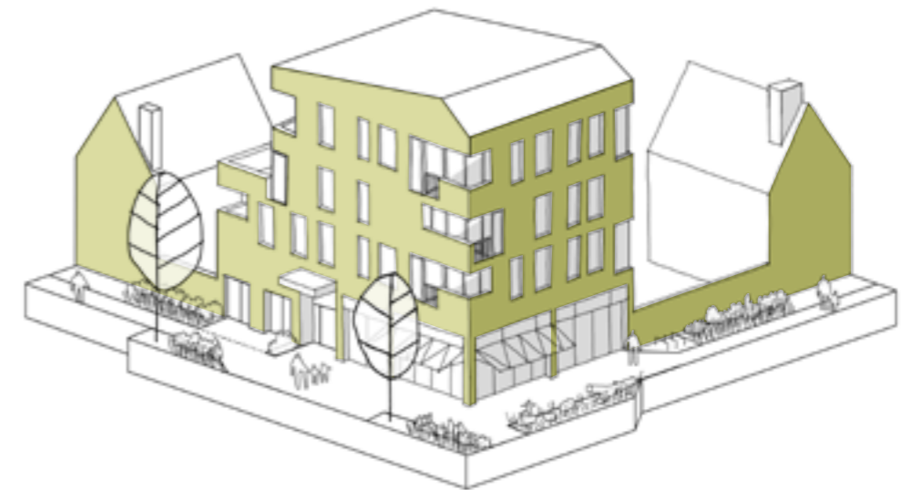
Fig 16: Site corners should always be given special consideration. Buildings should respond to their double frontage with windows, entrances and openings onto both street elevations.
